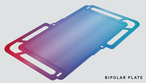
The image shows a metallic bipolar plate, which is a core element within the fuel cell system. Layered in stacks, bipolar plates provide the hydrogen and oxygen supply to the cells and distribute the coolant. Find out more in the article entitled »Cell growth« in our magazine
